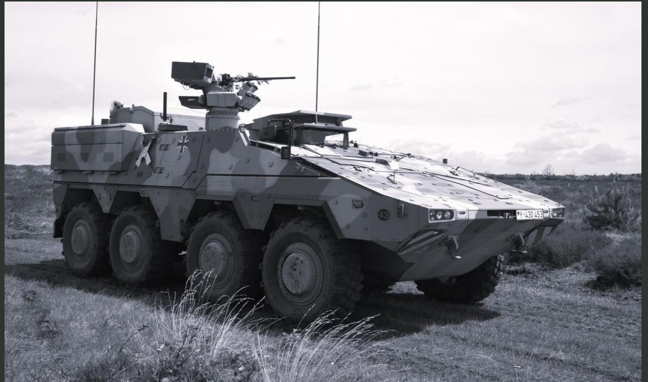
The Boxer is a modular wheeled armored vehicle consisting of a drive module and a mission module. The mission module has 28 variants.
